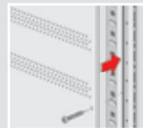
Fix to the upright with screws
