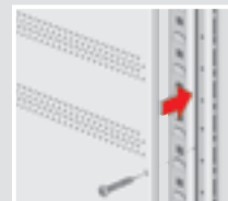
Fix to the upright with screws
